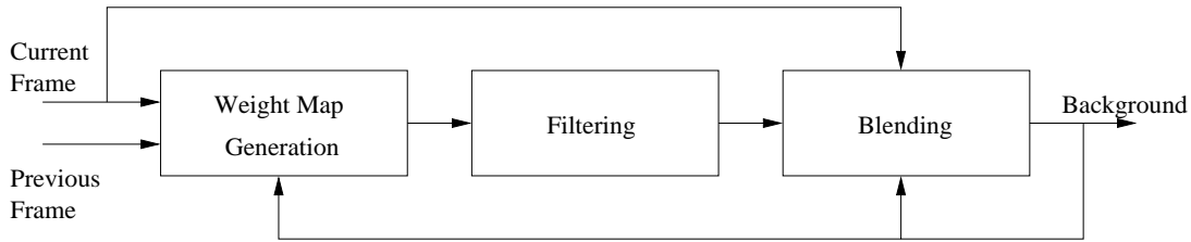
Figure 2: Block diagram of the iterative background adaptation. A background frame is generated by integrating information from the previous frame of the sequence and the already computed background.
