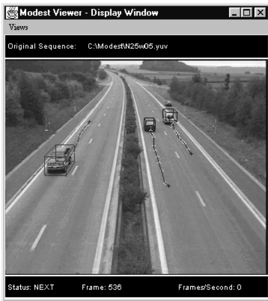
Figure 6: Example of final result of the MODEST system. The moving objects are tracked and their 3D shapes are described.
