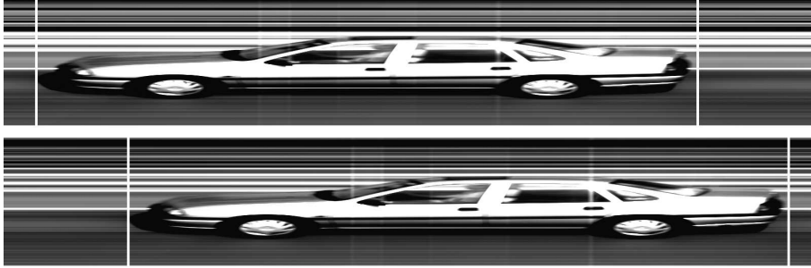
Figure 1.14: The detected boundaries of the vehicle. Overestimation of the length due to shadow is clearly visible in the front of the vehicle.
