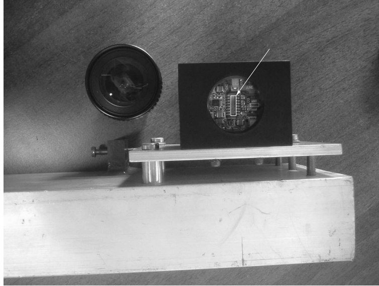
Figure 1.8: The camera pan/roll bases. The linear shape of the CCD is visible in the camera.
