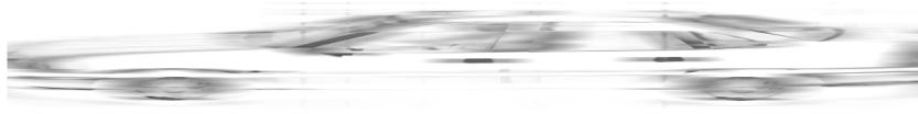
Figure 1.15: The feature map for the vehicle of fig.1.14: dark pixels correspond to featured areas
