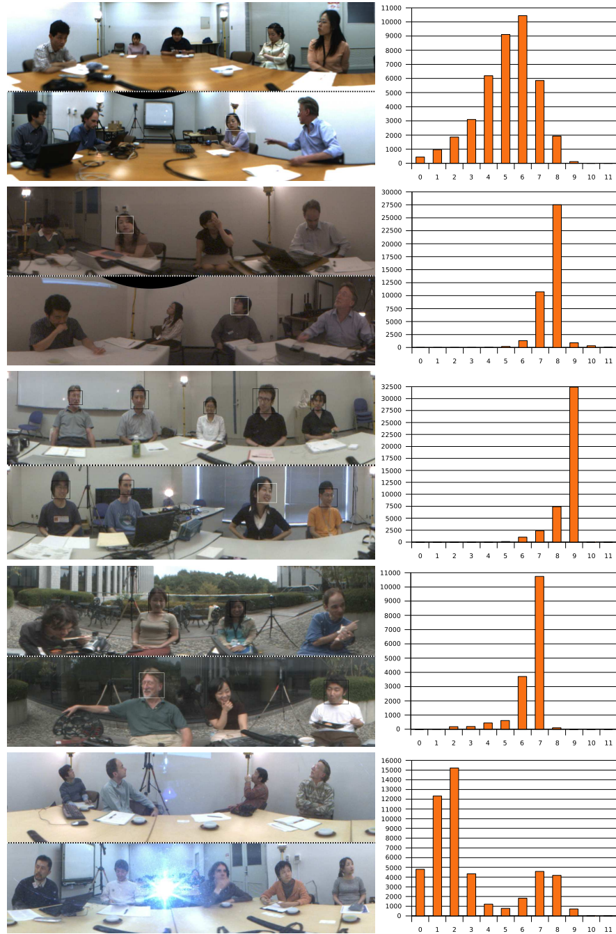
Fig. 6. Detection results for five test sequences. A representative image from the sequence is shown in the ( left column ). The ( right column ) contains the histogram of the number of images ( vertical axis ) per number of people detected ( horizontal axis ).
