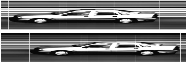
Fig. 3. The detected boundaries of the vehicle. Overestimation of the length due to shadow is clearly visible in the front of the vehicle.
