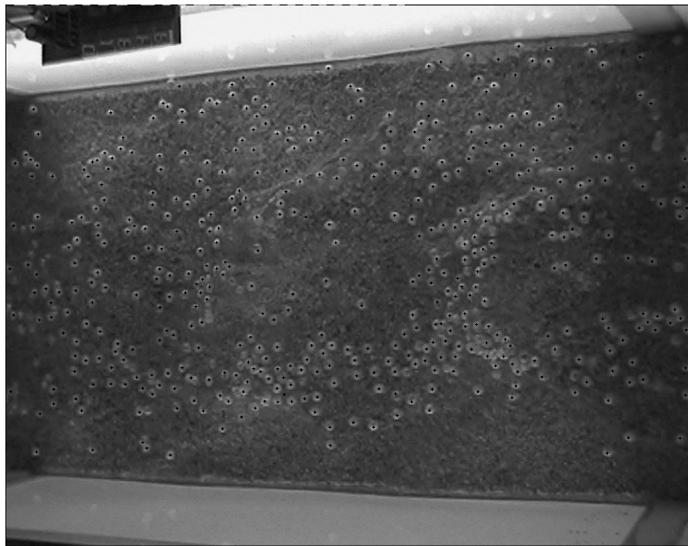
Figure 6.10: After the elimination of false particles on the flume armatures, only points in the fluid part of the scene remain.
